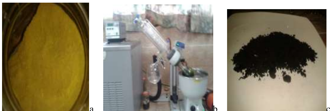
Figure 2: a. Powder of leaves of Annona muricata , b. Evaporation with ROTA VAPOR, c. Extract obtained
